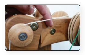
Loosen the jcb bolt from behind the spinning head. Move the head up in the slot until the white Dacron belt is tight and then, using the 4mm allen key provided, and working from the rear, tighten the head into position. This will be approximately at the central location in the slot.
