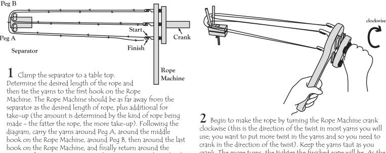
outside of Peqs B and A, ending where you began. There should be two lines of yarn from each peg. For a thicker rope, repeat the process as many times as desired.
