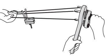
**3** Now twist the three strands together to make a rope. Take hold of the yarns at the back of the separator. Hold the three strands and pull them slowly away from the separator, twisting them together in a counter-clockwise direction (opposite what you did in the first step). It is helpful to have a second person hold the Rope Machine while you pull the yarn through the separator. Add more twist, if needed, by cranking clockwise.
