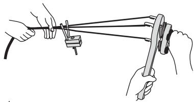
4 The three strands will naturally twist together. As you pull them through the separator, guide the yarns to ensure that they are even and smooth. As the Rope Machine moves closer and closer to the separator, occasionally give the crank a few clockwise turns to keep the strands tightly twisted. When the Rope Machine reaches the separator, slip the three strands off the hooks and tie an overhand knot in the end to prevent raveling.
