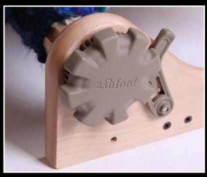
To advance the warp when weaving - turn the back handle slightly, lift the pawl out of the teeth, advance your warp and click the pawl back into the teeth.
